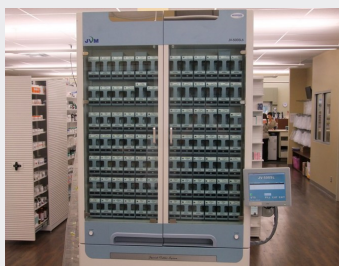
Automated unit dose machine for AUD medication packaging is located at Vancouver General Hospital.
